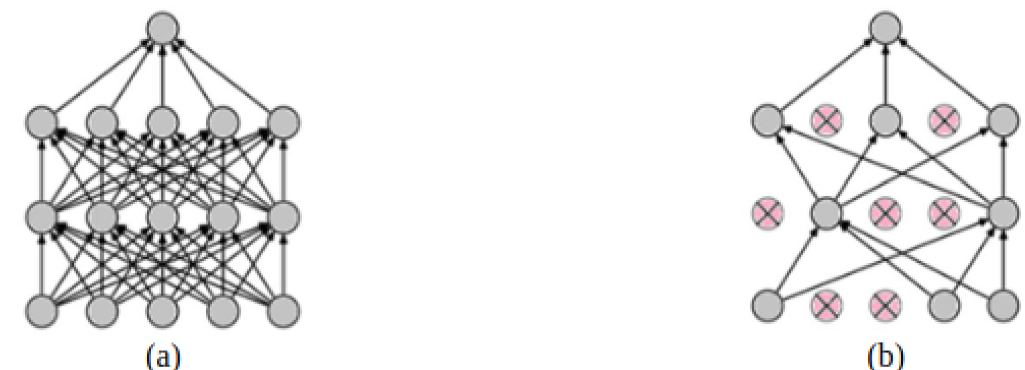
Figure 3: Applying dropout to prevent neural networks from overfitting (a) standard neural net and (b) after applying dropout
