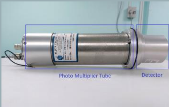
EJ-301 liquid scintillation detector and photo-multiplier tube [1]
