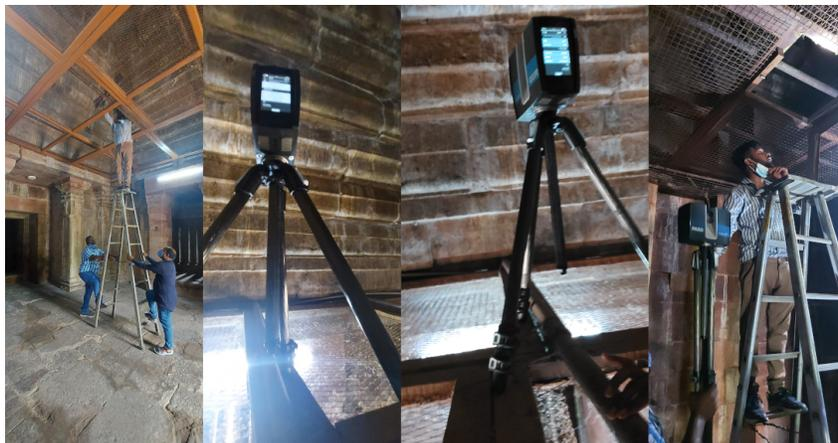
Figure 8: Scanning with an obstruction with ASI installed grill on the ceiling.
