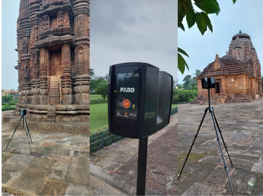
Figure 7: Terrestrial laser scanner.
