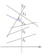
• Sweep line reaches right endpoint of a line segment: delete the line segment
