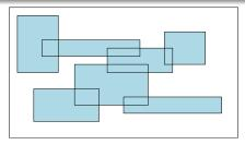
• Given a layout in which objects are orthogonal polygons with sides parallel to the axises. The task is to find the area covered by all the objects.
