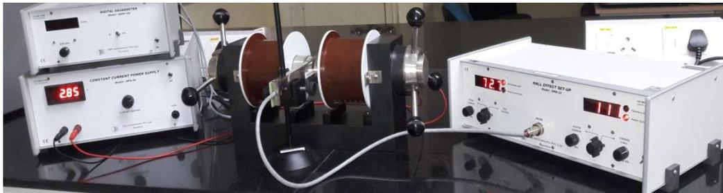
**Fig. 7: Set up for Hall voltage measurement**
