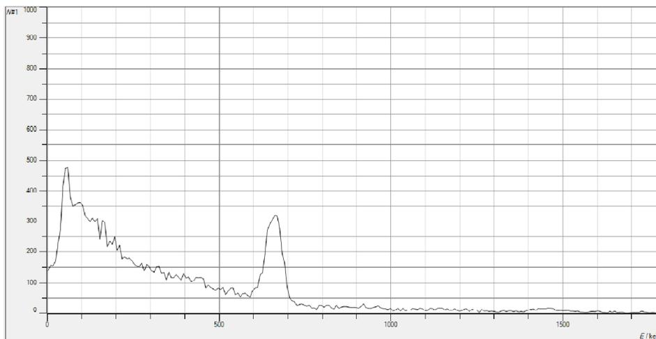
**Fig. 3: A typical gamma ray spectrum obtained for Cs-137 after calibration**
