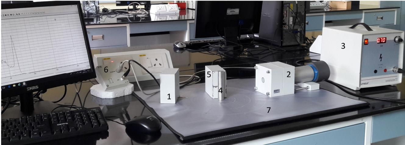
**Fig 2. Experimental set up for Compton scattering experiment consisting of Source holder, Scintillator detector with lead shielding, High voltage supply, Scatterer, Additional movable shielding, MCA and a Experimental panel with angular scale (shown respectively as nos. 1-7)**
