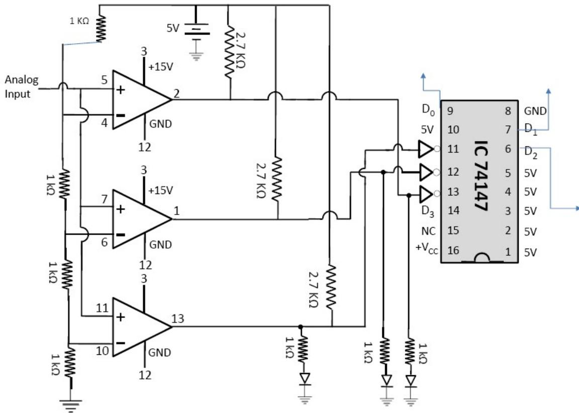
Figure 2. Circuit diagram for 2 bit binary Analog to Digital conversion
