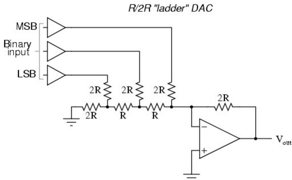
Figure 1. Circuit diagram for digital to analog conversion
