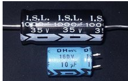
Fig. 2: Axial and Radial Electrolytic capacitors
