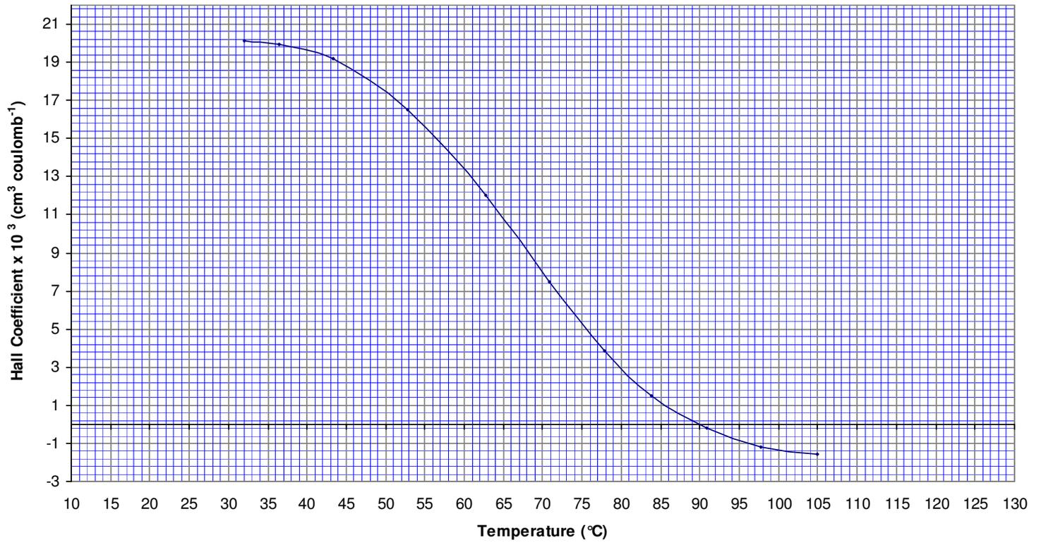
**Fig. 8: Sample graph showing Hall coefficient ~ Temperature for p-Ge**
