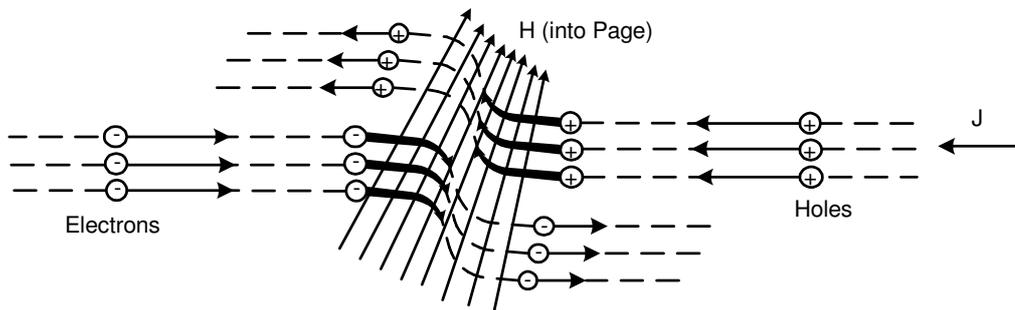
Fig. 1 Carrier separation due to a magnetic field
