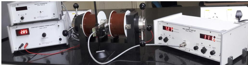
**Fig. 7: Set up for Hall voltage measurement**
