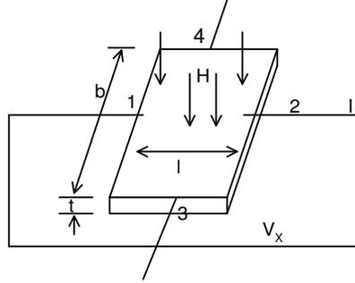
**Fig. 4 Schematic arrangement for the measurement of Hall Effect of a crystal**
