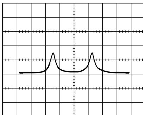
Fig. 8 Line Sketch of the Resonance Peak
