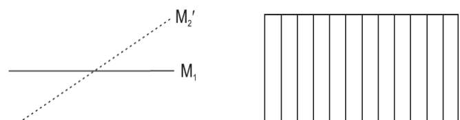
Fig. 4: Formation of straight line fringes
