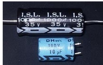
**Fig. 2: Axial and Radial Electrolytic capacitors**
