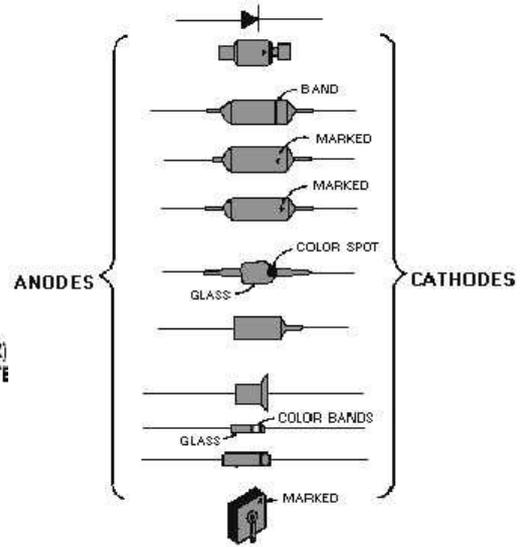
**Fig. 4: Identification of Diode**
