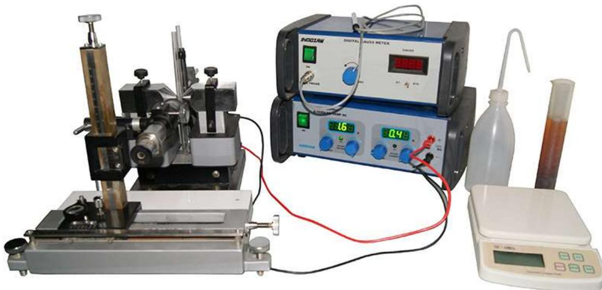
Fig. 2 Experimental set up for Quincke's method
