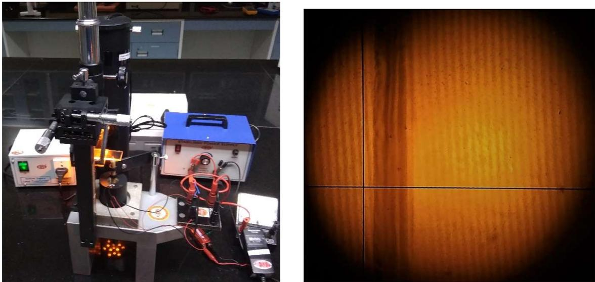
**Fig. 4: Experimental set up and the Fizeau's fringes**
