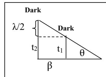
**Fig. 1: angle of wedge shaped air film**
