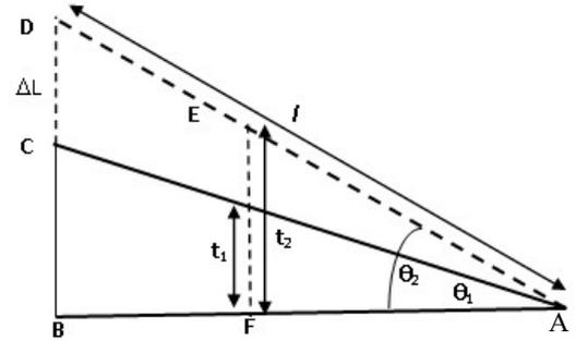
Fig. 2: Geometry to calculate the optical path difference
