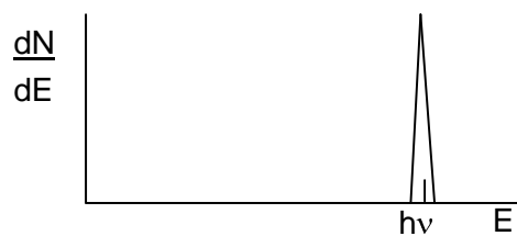
Fig. 2: Photopeak corresponding to photoelectron absorption events
