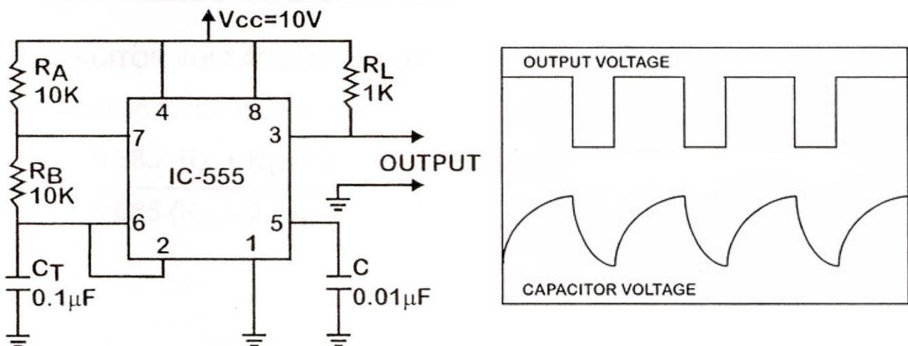
***Astable multivibrator with duty cycle less than 50%:***
