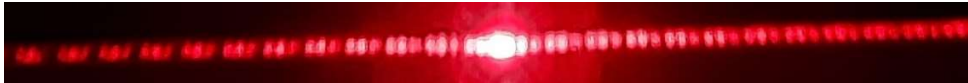
Figure 5. Photographic image of double-slit diffraction pattern – each diffraction maxima is broken up into interference fringes
