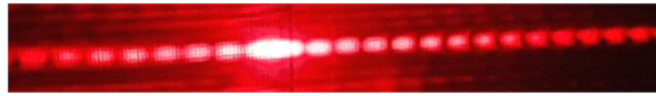
Figure 3. Photographic image of diffraction pattern from a thin wire – similarity with single-slit pattern is what Babinet’s principle asserts.
