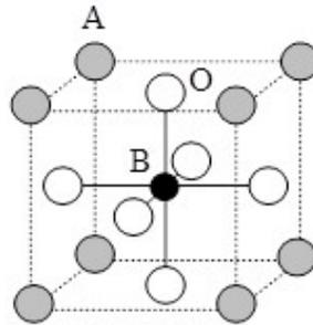
Figure 2 (a). Perovskite  $ABO_3$  structure with the A and B cations on the corner and body centre positions, respectively. Three oxygen anions per unit cell occupy the faces and form octahedra surrounding the B-site.
