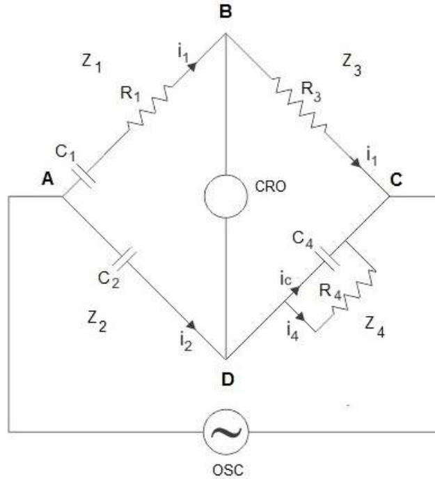
The figure above shows the configuration of the Schering Bridge, where,
