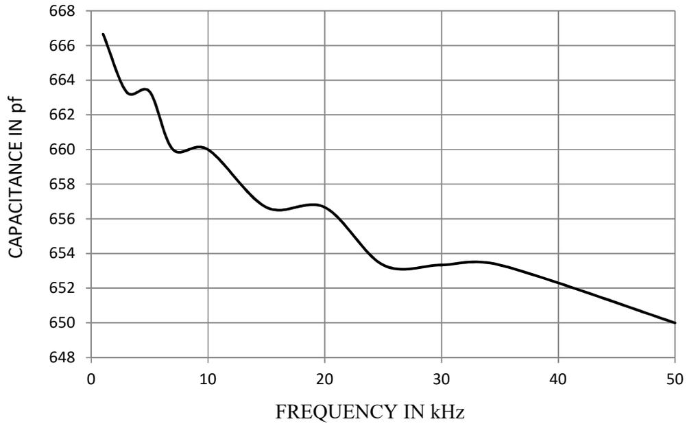
Fig. 11 Plot of Capacitance as a function of frequency (MLCC)
