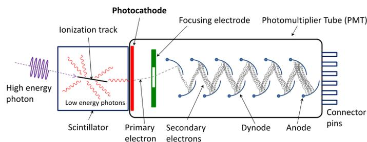
**Figure 1:** Schematic diagram of a photomultiplier tube. (By Qwerty123uiop, CC BY-SA 3.0, <https://commons.wikimedia.org/w/index.php?curid=62426194>)
