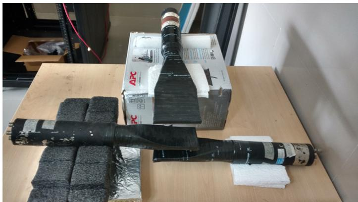
**Figure 3:** Arrangement of scintillator paddles.
