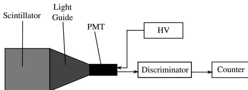
**Figure 2:** Circuit diagram for counting scintillator detector signals
