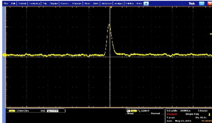
**Figure 7:** Signal after Spectroscopic Amplifier (Unipolar signal, 300 mV/div, 5.0  $\mu$ s/div, 50  $\Omega$  termination)
