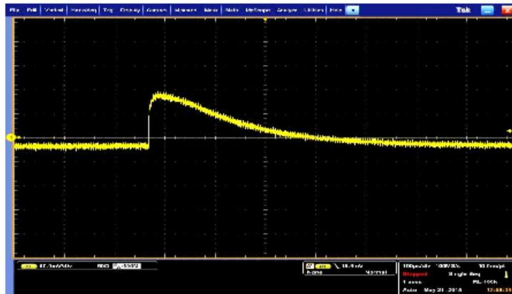
**Figure 6:** Signal after preamplifier (60 mV/div, 100  $\mu$ s/div, 50  $\Omega$  termination)
