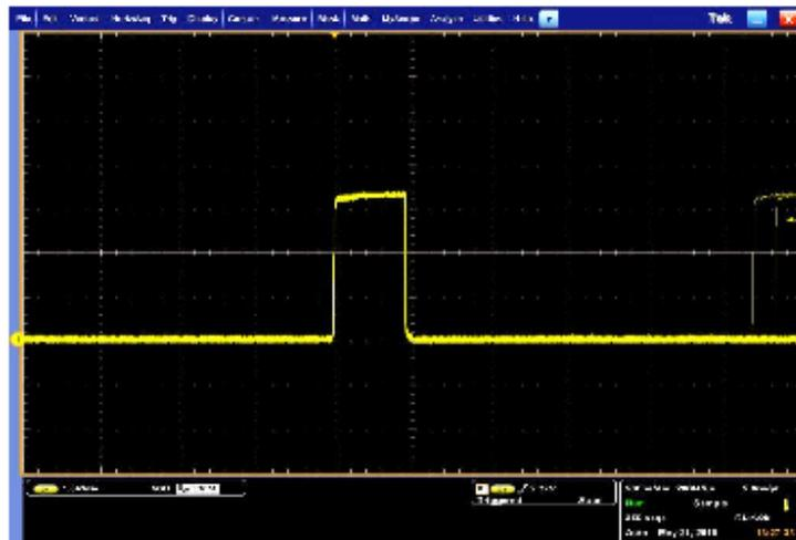
**Figure 8:** TTL Signal after SCA (Single Channel Analyser) (Digital signal, 1.0 V/div, 500 ns/div, 50  $\Omega$  termination)
