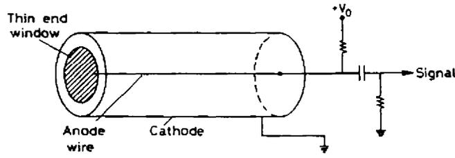
**Figure 1:** Basic configuration of a gas detector
