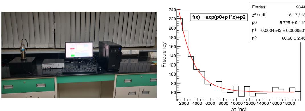
**Figure 1:** (a) Picture of the setup. (b) Decay spectrum obtained from the setup. The inverse of parameter ‘p1’ gives the mean lifetime of muon in nanoseconds.
