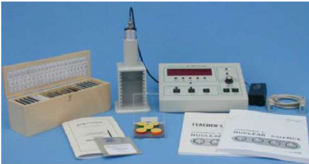
Fig. 1 Experimental set up for studying dead time and counting statistics
