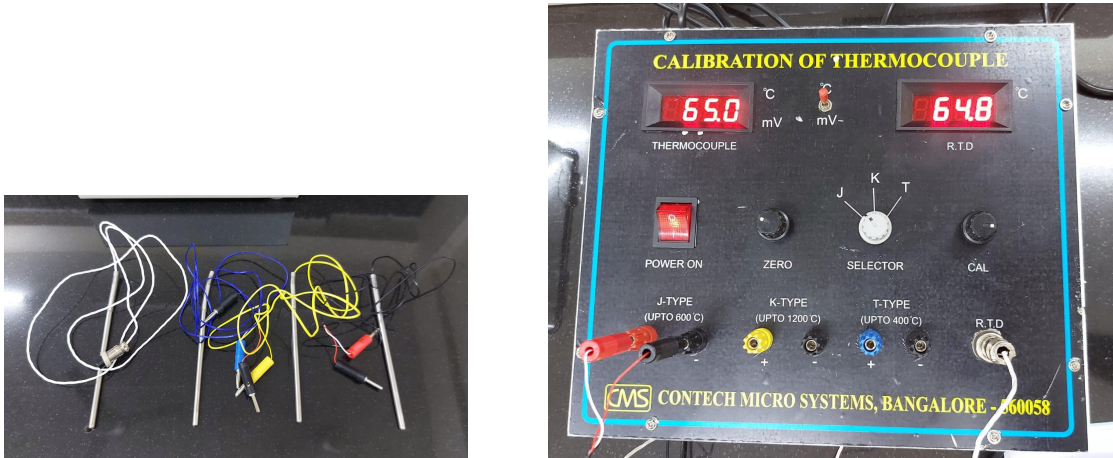
Fig. 1: Left: Photograph of the thermocouples showing probe (stainless steel sheath) and connection wire. Right: The Digital Temperature Indicator (DTI).
