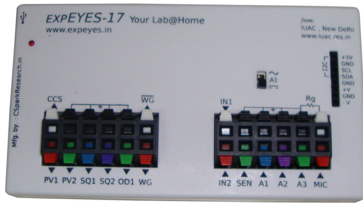
Figure 1.1: The ExpEYES17 top panel showing the external connections.
