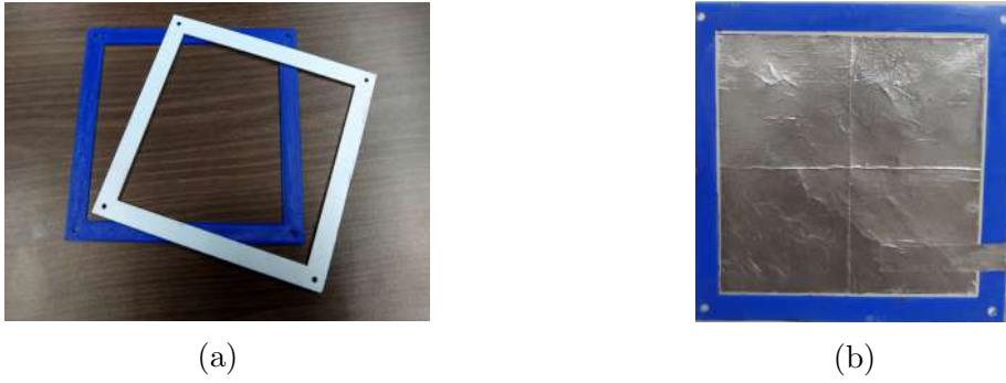
Figure 4.6: (a) The Perspex frame with the inlet and outlet valves. (b) The rubber layer that will be placed on top of the Perspex layer to act as a seal for the joint.
