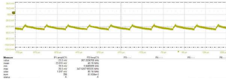
Figure 4.16: The preamplifier output for the the input pulse shown in Figure 4.15.
