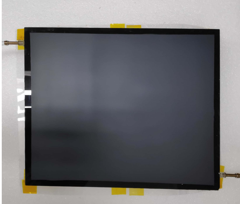
Figure 2.1: Resistive Plate with Graphite Coating
