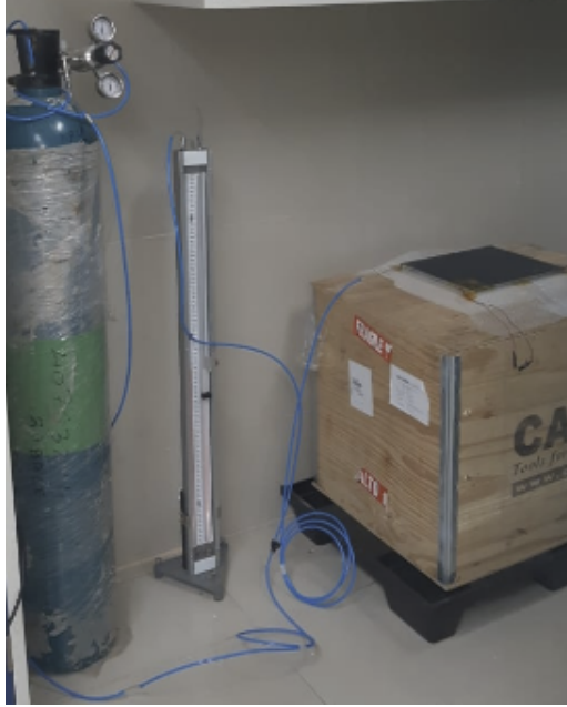
Figure 3.3: Apparatus for leak test
