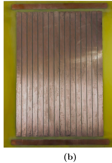
Fig. 3.11: (a) A 160 \times 160 \text{ mm}^2 glass RPC (b) A Printed Circuit Board (PCB) panel is used to develop 16 strips of copper read-out for reading the RPC signal.
