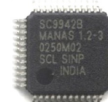
MANAS: 16 channel Amplifier, shaper, track and hold for ALICE
