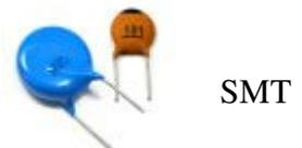
**Fig. 3: Ceramic capacitors**
