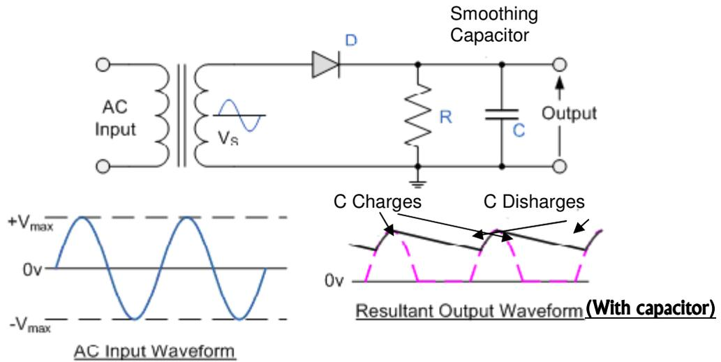
**Fig.2: Half-wave rectifier circuit with capacitor filter**
