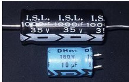
**Fig. 2: Axial and Radial Electrolytic capacitors**
