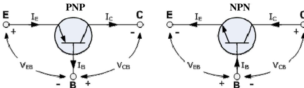
The symbols for both the NPN and PNP bipolar transistor are shown above along with the direction of conventional current flow. The direction of the arrow in the symbol shows current flow between the base and emitter terminal, pointing from the positive P-type region to the negative N-type region, exactly the same as for the standard diode symbol. For normal operation, the emitter-base junction is forward-biased and the collector-base junction is reverse-biased.
